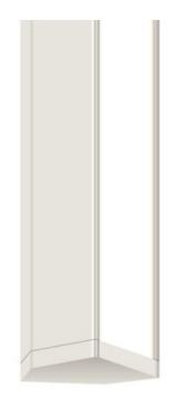
SHADE COLOR White **BODY FINISH** Satin Nickel WATTAGE DIMMER Low Voltage Electronic DIMENSIONS 13"L x 1.4"W x 1.37"D INTEGRATED LED MODULE LAMP LED/7W/12V LED Technical Information LUMINOUS FLUX 286 lumens LUMENS/WATT 40.86 LAMP COLOR 2700K COLOR RENDERING 92 CRI
