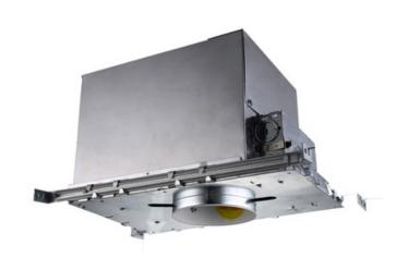
TRIM COLOR N/A BODY FINISH Galvanized Steel WATTAGE 50W DIMMER Low Voltage Magnetic DIMENSIONS 14.9"W x 7.1"H **BULB NOT INCLUDED** LAMP 1 x MR16/GU5.3 (bipin)/50W/12V Halogen 1 x MR16/GU5.3 (bipin)/12V LED Technical Information CEILING TYPE Drywall with Trim HOUSING TYPE New construction IC Airtight HOUSING HEIGHT
