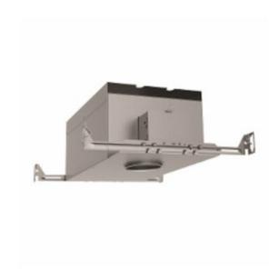
BODY FINISH Galvanized Steel WATTAGE 35\// DIMMER Low Voltage Electronic DIMENSIONS 15.25"L x 8.25"W x 7.9"H **BULB NOT INCLUDED** LAMP 1 x MR16/GU5.3 (bipin)/35W/12V Halogen MR16/GU5.3 (bipin)/12V LED Technical Information CEILING TYPE Drywall with Trim HOUSING TYPE New construction IC Airtight HOUSING HEIGHT APERTURE SIZE 3.500"
