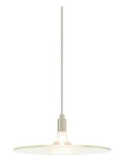
SHADE COLOR Clear BODY FINISH Satin Nickel WATTAGE 50W DIMMER Dimmable DIMENSIONS 72.1"L x 6.3"W x 0.1"H **BULB NOT INCLUDED** LAMP 1 x MR16/GU5.3 (bipin)/50W/12V Halogen
