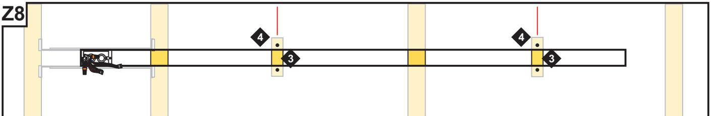
2: Cut 1" thick by 3" long sections of 2x4 to use as support bars.
