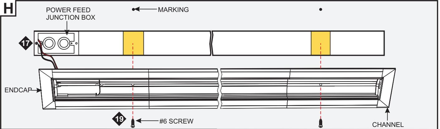
**17:** Insert the power wires into the channel end cap.
