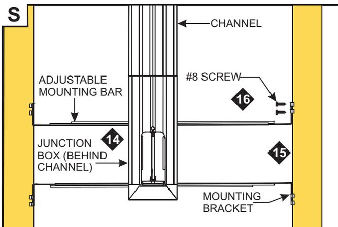
**14:** Align the junction box behind the mounted vertical channel section using the adjustable mounting bars and mount junction box to channel with the provided screw.
