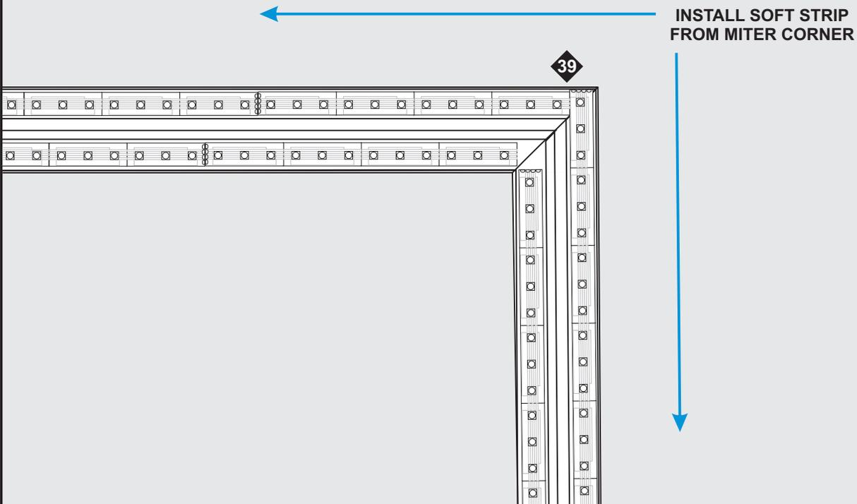
**NOTE:** Carefully measure the Soft Strip going inside the channel from the miter cut point toward the electrical boxes. Make sure the strip is no more than 2.4" longer than the channel section. Cut the Soft Strip at the marked cut points only. Refer to Soft Strip installation instructions for more details.
