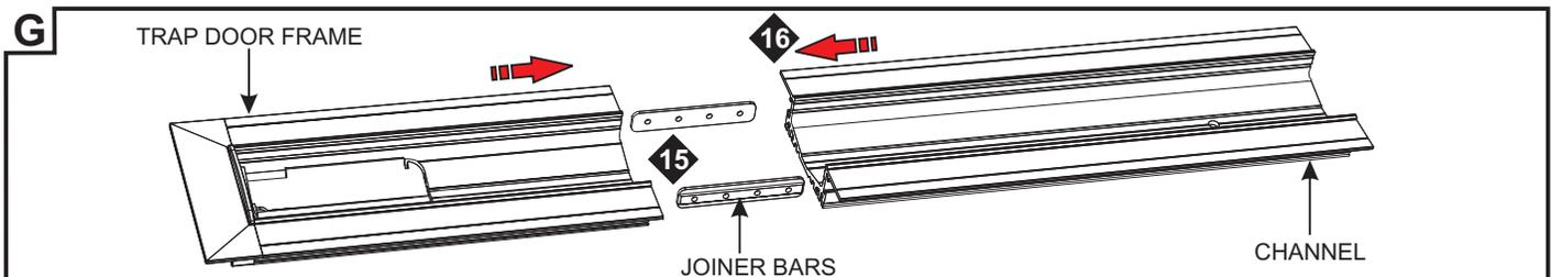
**15:** Insert the joiner bars halfway into the channel trap door frame. Tighten the two #4-40 set screws on each joiner bar with a 0.05" Allen wrench.
