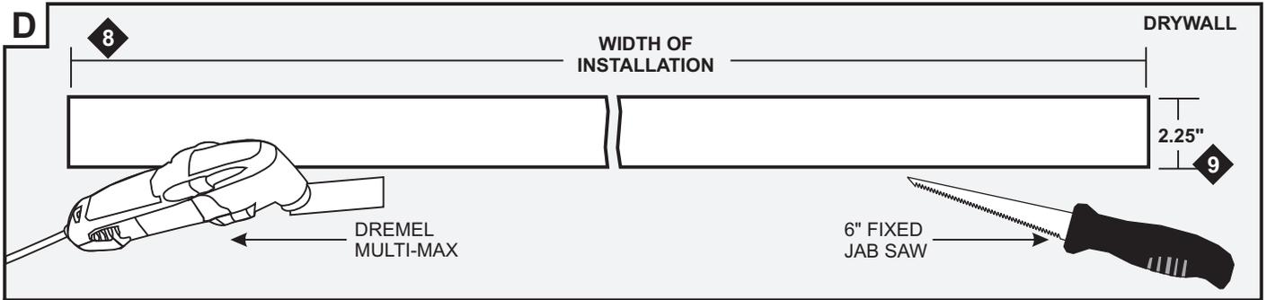
**8:** Mark the area where the channel will be located on the drywall.
