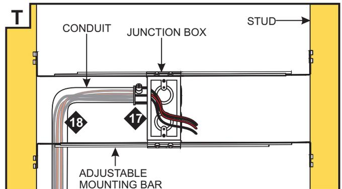
**17:** Remove a knockout to install the power line conduit.
