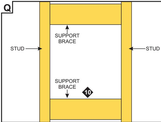
**10:** Cut and install 2x4 support braces between studs to support the channels as needed. Maximum recommended spacing between the support braces is 36".
