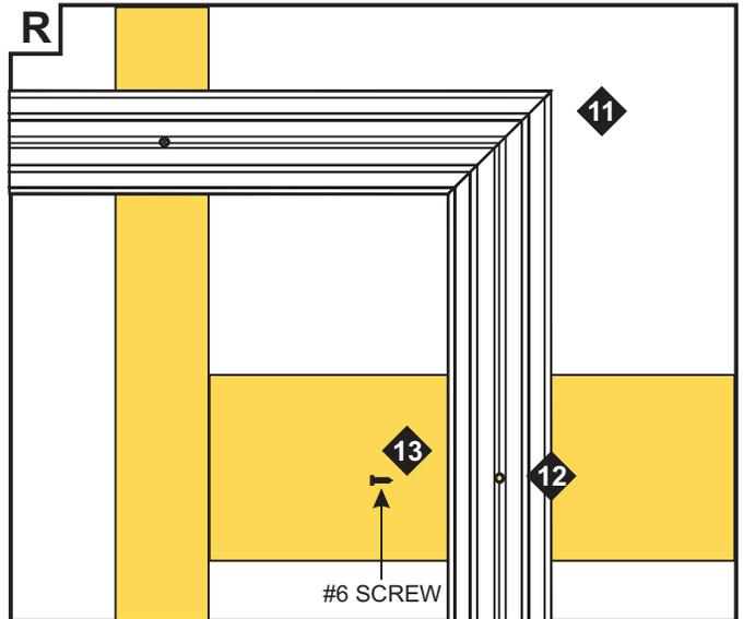
**11:** Align miter cut channel ends. Make sure there is no visible gap where miter corners meet.
