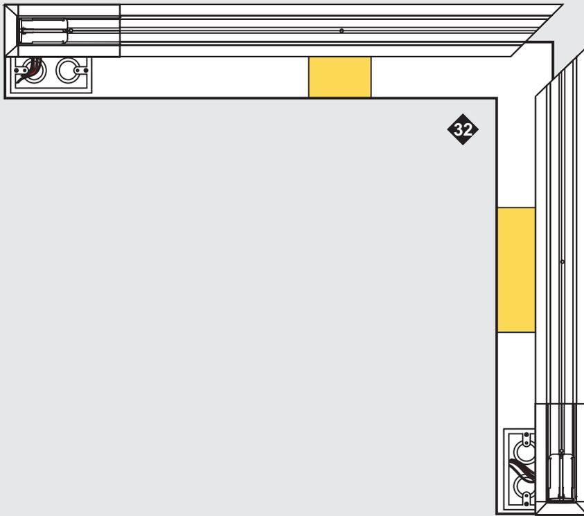
32: Reinstall both channel sections to junction boxes and studs/support braces by following Steps 8-9 on Page 5 and Steps 12-14 on Page 7.
