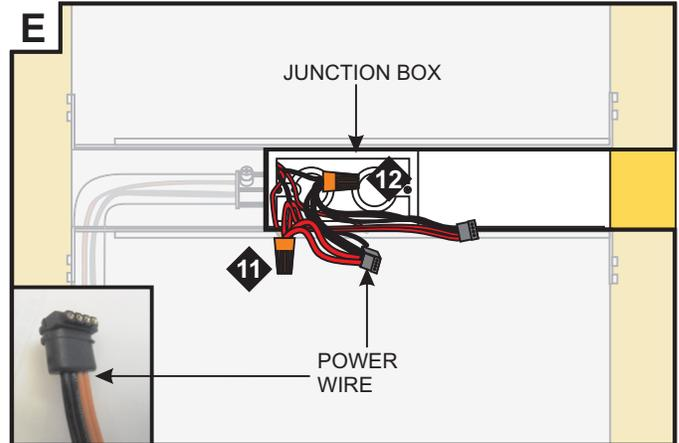
**11:** Connect the red power supply (24VDC+) wires to each red power wire with a wire nut inside the junction box.
