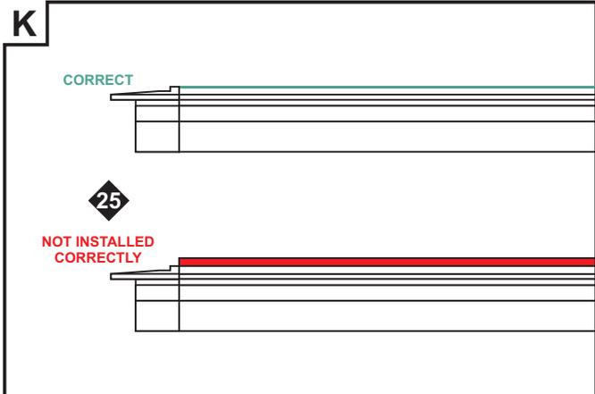
**25:** Snap the lens back onto the channel.
