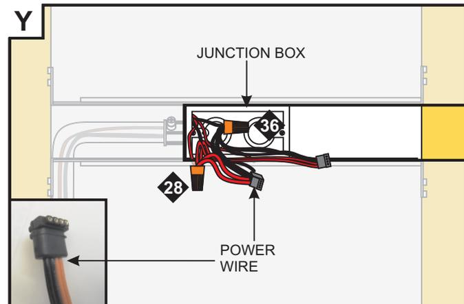
**27:** Connect the red power supply (24VDC+) wires to each red power wire with a wire nut inside the junction box.
