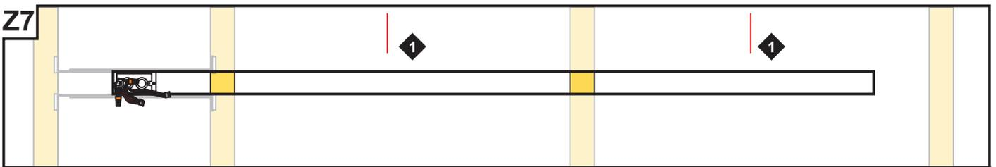
1: Mark the wall where channel mounting holes are located along the channel opening.
