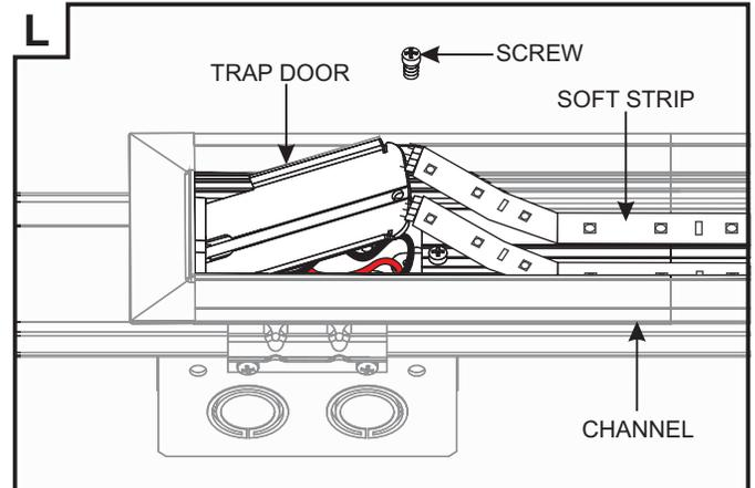
**NOTE:** If necessary access the wire connections by opening the trap door. Disconnect the soft strip and remove screw on the trap door. Pull open the trap door to expose the wiring.
