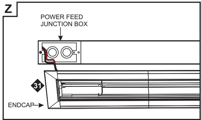
**31:** Insert the power wires into each channel end cap.
