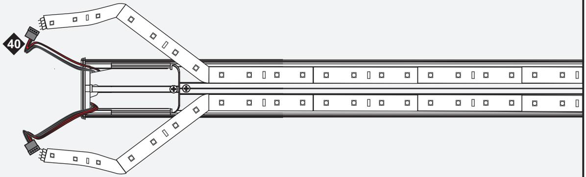
40: Line up the red wire side of the power connector with the “+24VDC” marking on the Soft Strip. Push the male connector of the Soft Strip into the female connector of the power cables.
