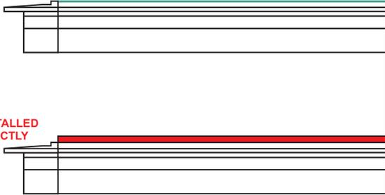
43: Snap the lens back onto the channel.
