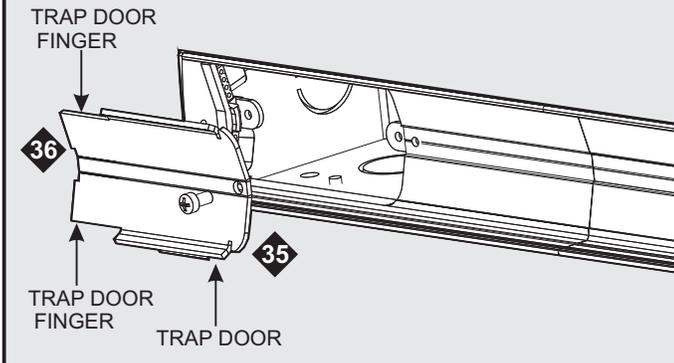
**35:** Remove the screw from the junction box and remove the trap door.
