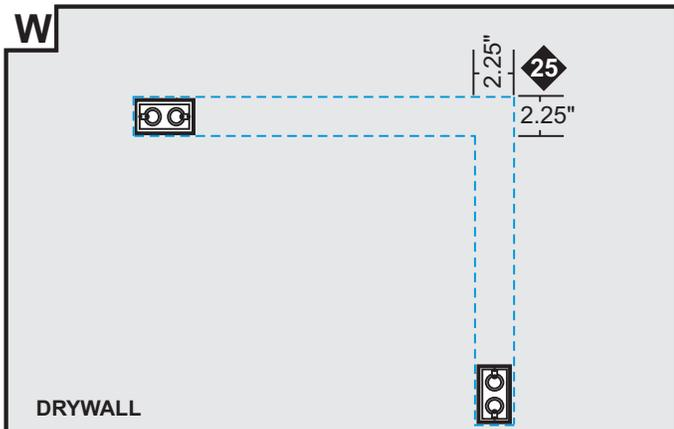
**25:** Mark the areas on the drywall where the channel will be installed.
