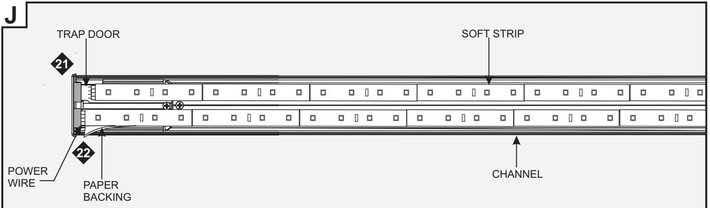
**22:** Line up the red wire side of the power connector with the "+24VDC" marking on the Soft Strip. Push the male connector of the Soft Strip into the female connector of the power cables.
