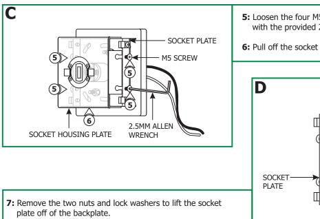
**5:** Loosen the four M5 screws on the sides of the socket plate with the provided 2.5mm Allen wrench (**Do Not Remove**).
