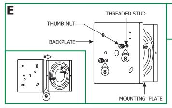
**NOTE:** The mounting plate and backplate can be omitted for indoor locations only if socket plate covers the entire electrical box.
