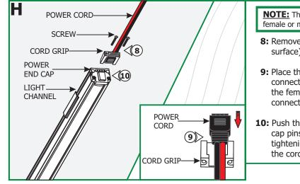
**NOTE:** The power feed cable can be mounted to either the female or male end of the channel.
