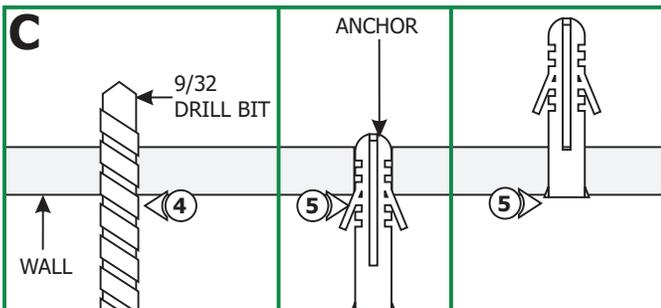
**4:** Use a 9/32 drill bit to make holes on all six marked points.
