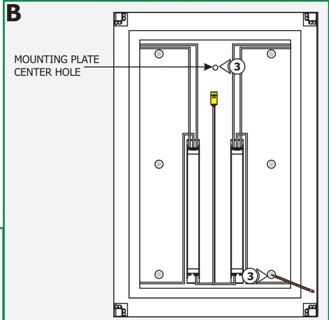
**3:** Align the mounting plate hole with the power line conduit, or electrical box, and use the mounting plate as a template to mark four mounting holes onto the wall.
