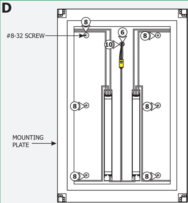
**6:** Install the conduit connector (not provided) to mounting plate hole. Feed the power line through the conduit connector into the mounting plate.
