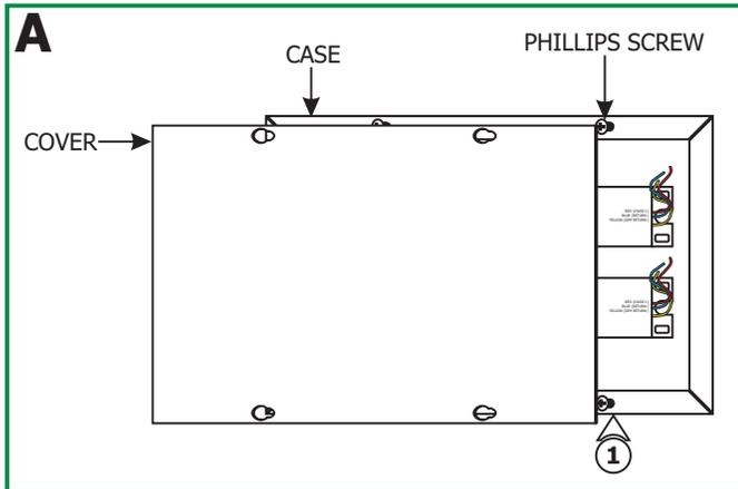
**1:** Loosen the four Phillips screws on the front of the power supply cover to slide the cover off of the case.
