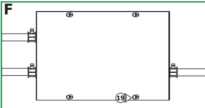
**19:** Replace the power supply cover and secure it by tightening the four Phillips screws.
