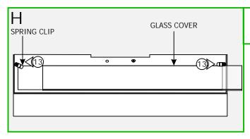
13: Loosen the screws on the spring clips (Do Not Remove) to insert the glass cover under the clips. Slightly tighten the spring clip screws to secure the glass cover in place.
