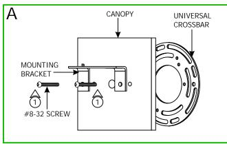
1: Loosen the two #8-32 screws from the canopy to remove the universal crossbar.
