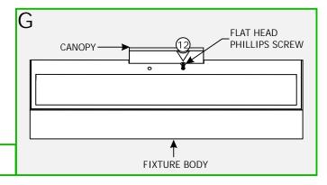
12: Secure the right fixture body hole with the flat head Phillips screw provided.
