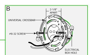
2: Mount the universal crossbar to the electrical box holes with the provided #8-32 screws so that the two inner threaded holes (spaced 2-1/8" apart) on crossbar are leveled horizontally.
