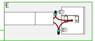
9: Connect each power supply wire to a fixture body wire (either one) with a wire nut.
