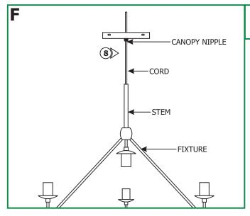
**8:** Feed the fixture cord into the canopy and secure the canopy to the stem by tightening the canopy nipple completely into the stem.
