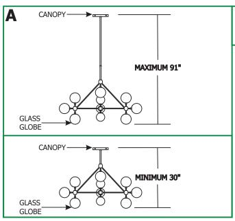
**NOTE:** Determine the desired overall fixture height using the 8" stem only or using additional combination of 20" and 12" stems for a maximum overall height of 91".
