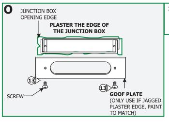
**13: Optional:** Use the Goof Plate if the junction box opening has a lot of imperfection/jagged edges. Install the provided goof plate (paint to match prior) with the two screws.
