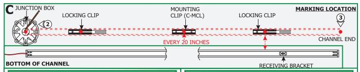
**NOTE:** Remote power supply must be installed within 40ft of Junction box. The low voltage 24V DC wires must be present in Junction box before installing the channel. Refer to the installation instructions provided with the power supply. See page 5 for wiring diagram.
