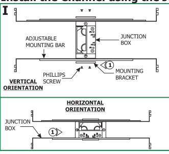
**1:** Mount each adjustable mounting bar to one side of the junction box (mounts to any side of the housing depending on the orientation of the channel) and secure them with the mounting brackets and two Phillips screws provided.
