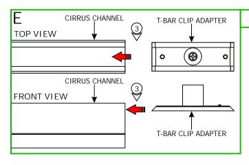
4: Align the T-bar clip adapters evenly apart and tighten the #6-32 set screws on each T-bar clip adapter with a 1/16" Allen wrench.
