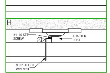
7: Replace the end cap to the end of the channel and tighten two #4-40 set screws with a 0.05" Allen wrench.
