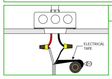
11: Insert all wires into junction box and mount the cable grip assembly to the 2" Plaster Ring using two #8-32 screws.
