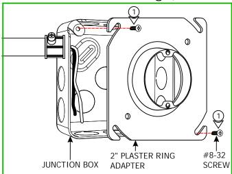
NOTE: Junction box must be mounted to allow clearance of ½" between the face of the junction box and the drywall surface.
