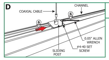
**6:** Carefully move the sliding post to the predetermined location on channel and tighten the #4-40 set screw on the sliding post bed with the 0.05" Allen wrench.
