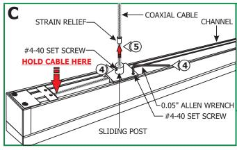
**WARNING:** To avoid damaging the coaxial cable electrical connection, make sure that the end of the coaxial cable coming out of the fixture is held with thumb before relocating sliding posts.
