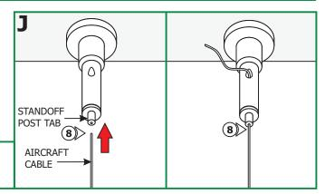
**8:** Push the tab on standoff while feeding the aircraft cable coming from the channel into a standoff so that it holds one end of the fixture in place.
