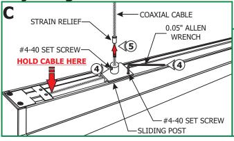
**WARNING:** To avoid damaging the coaxial cable electrical connection, make sure that the end of the coaxial cable coming out of the fixture is held with thumb before relocating sliding posts.
