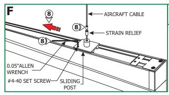
**8:** Repeat Steps 4 through 7 for aircraft cable side. Note that there are two intermating strain relief tubes.
