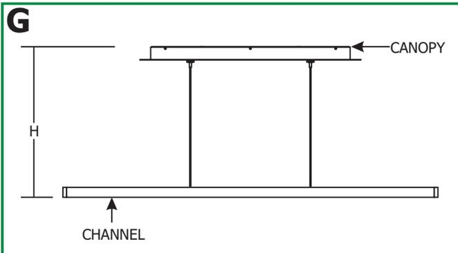
**NOTE:** Determine the fixture height (H), from the bottom of the channel to the top of the canopy.
