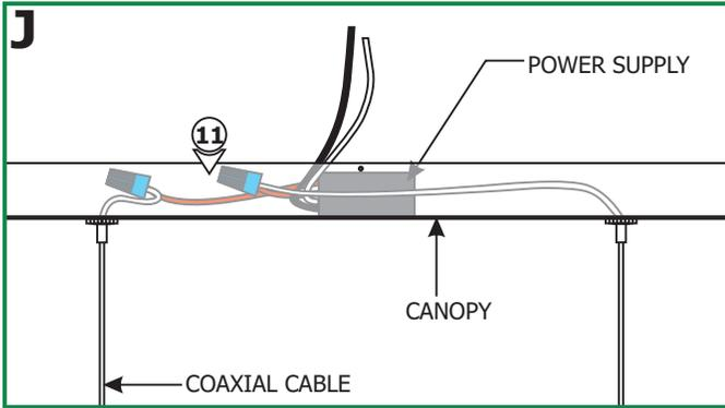
**11:** Connect each coaxial cable bare wire to the low voltage red power supply wires with a wire nut.
