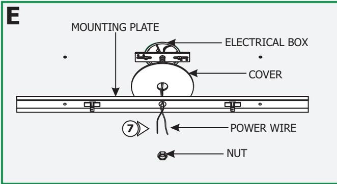
**7:** Slide the cover and mounting plate center hole onto the crossbar threaded nipple and secure it with the nut provided.
