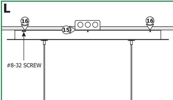
**15:** Place all the wires and wire nut connections inside the canopy.
