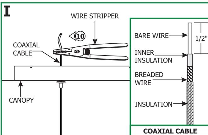
**10:** Use the #16 gauge hole of the AWG wire strippers to strip 1/2" of the insulation along with braided wire and inner wire insulation.
