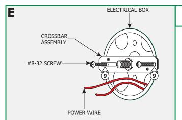
**9:** Mount the crossbar assembly to the electrical box holes with the provided #8-32 screws.
