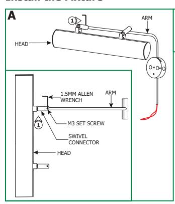
1: Rotate the Cody's head perpendicular to the arm making sure the arm is completely inserted into the head swivel connector. Tighten the M3 set screw on the swivel connector with the provided 1.5mm Allen wrench to secure the head in place.
