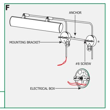
**10:** Line up the mounting bracket holes with the anchors and secure the fixture to the anchors with the four #8 screws provided.
