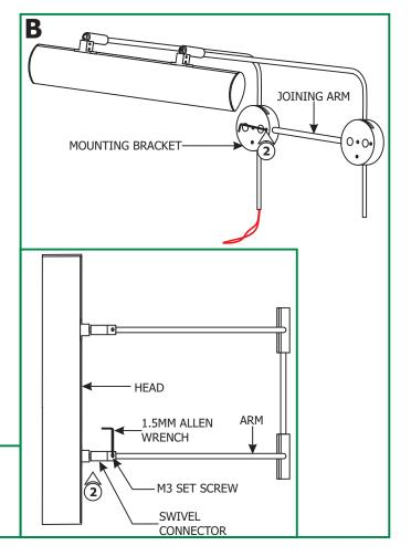
2: Insert the loose arm assembly (provided in the box) into the other swivel connector, insert the joining arm into the mounting bracket of the first arm. Tighten the M3 set screw on the swivel connector and mounting bracket with the 1.5mm Allen wrench.
