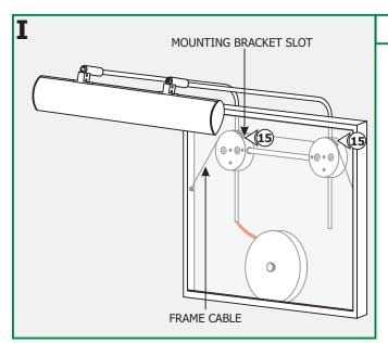
**15:** Hang the frame cable into the two mounting bracket slots.
