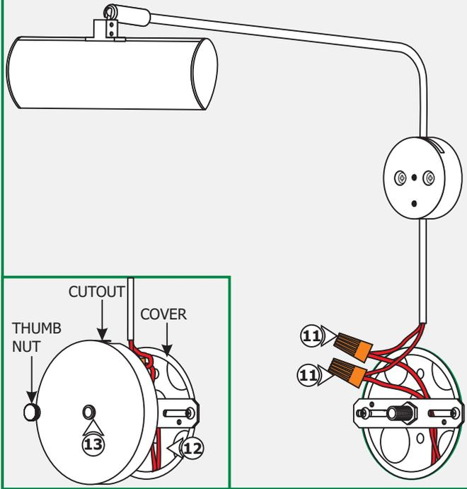
**11:** Connect each low voltage LED power supply wire (red wire) to one fixture wire with a wire nut.
