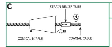
**4:** Feed the coaxial cable through the conical nipple and flared side of the strain relief tube. Slide the conical nipple and strain relief tube down the coaxial cable.
