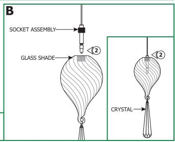
**2:** Gently place the glass shade onto the socket assembly. Rotate the glass shade to secure it to the socket thread until the top of the socket thread is flush with the glass shade.
