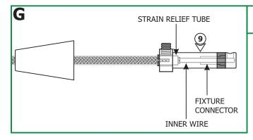
**9:** Feed the inner coaxial cable along with strain relief tube into the coaxial fixture connector.
