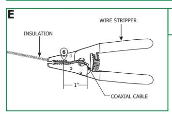
**6:** Use the #12 gauge hole of the AWG wire strippers to strip 1" of the insulation cover from the end so that the bare coaxial cable is exposed.
