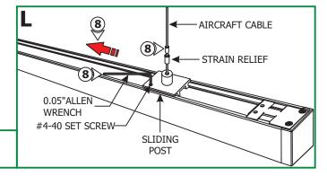
**8:** Repeat Steps 4 through 7 for aircraft cable side. Note that there are two intermating strain relief tubes.
