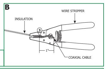
**3:** Use the #12 gauge hole of the AWG wire strippers to strip 1" of the insulation cover from the end so that the bare coaxial cable is exposed.
