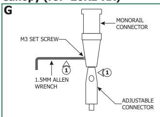
**NOTE:** Make sure the Fast Jack Canopy is installed. One of the Fast Jack ports will be used as a support post and the other will power the fixture. The center distance between the Fast Jack ports is 14". Depending on the fixture length, the coaxial and aircraft cable posts on the fixture will need to be moved towards the center so that they are 14" apart.
