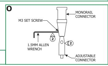
2: Loosen the M3 set screw on the adjustable post with the 1.5mm Allen wrench to remove the adjustable connector from the Monorail connector.
