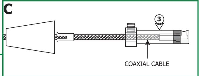
**3:** Feed the coaxial cable into the coaxial fixture connector. The coaxial cable will come to a stop point.
