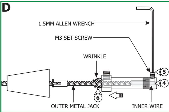
**4:** Keep feeding the coaxial cable in until the inner wire is visible in the screw hole of the fixture connector tip. The outer metal jacket will start to wrinkle.
