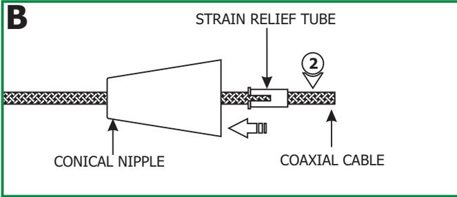
**2:** Feed the coaxial cable through the conical nipple and flared side of the strain relief tube. Slide the conical nipple and strain relief tube down the coaxial cable.
