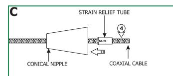
**4:** Feed the coaxial cable through the conical nipple and flared side of the strain relief tube. Slide the conical nipple and strain relief tube down the coaxial cable.
