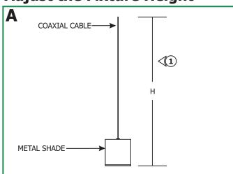
1: Cut the coaxial cable to the desired height (H) with a sharp cutter. The overall fixture height is measured from the bottom of the metal shade to the end of the coaxial cable.
