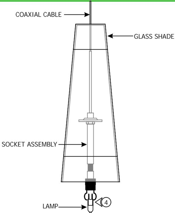
**CAUTION:** To reduce risk of a burn or electrical shock during lamping, disconnect the power to the fixture.
