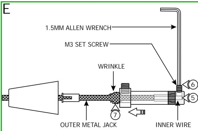
5: Keep feeding the coaxial cable in until the inner wire is visible in the screw hole of the fixture connector tip. The outer metal jacket will start to wrinkle.
