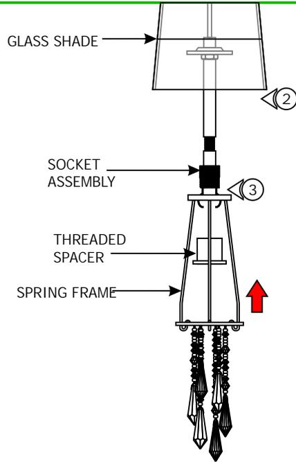
2: Lift the glass shade up, to expose the socket assembly.
