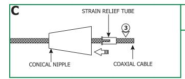
**3:** Feed the coaxial cable through the conical nipple and flared side of the strain relief tube. Slide the conical nipple and strain relief tube down the coaxial cable.
