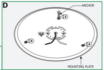
**4:** Mark the three mounting plate holes on the ceiling.
