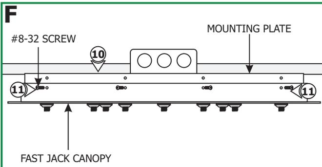
**10:** Place all wires and wire nut connections inside the canopy.
