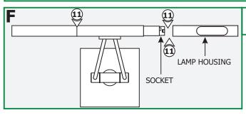
**11:** Pull out the two lamp housings from the fixture to expose the two sockets.
