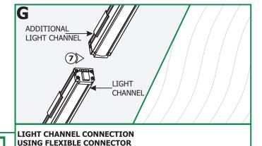
**NOTE:** Multiple light channel can be connected together directly by connecting male end of one to the female end of the other one, or by using the flexible connectors up to a maximum of 25 feet.
