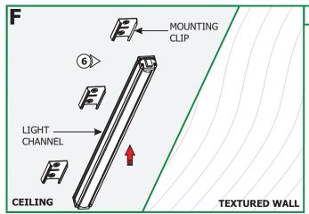
**6:** Snap each Light Channel into the spring clips.
