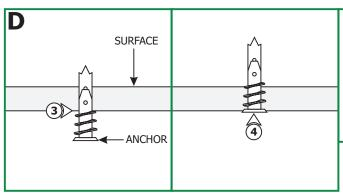
**NOTE:** Steps 4 to 6 are for drywall mounting. Omit these steps if mounting the clips to a wood surface directly. **ANCHORS ARE NOT PROVIDED.**
