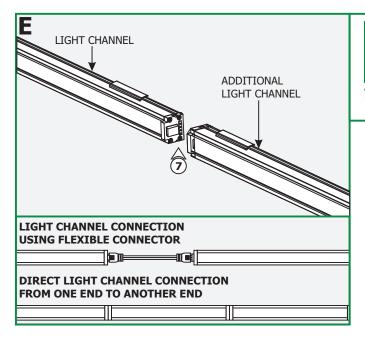
**NOTE:** Multiple light channel can be connected together directly by connecting male end of one to the female end of the other one, or by using the flexible connectors up to a maximum of 25 feet.
