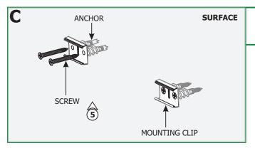
**5:** Line up the mounting clips to the anchors and secure it to the anchors by tightening the two #8-32 screws to each clip.
