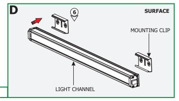
**6:** Snap each Light Channel into the spring clips.
