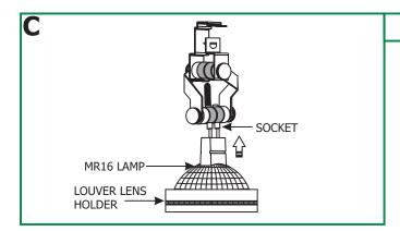
**6: (OPTIONAL)**-For fixtures like Gear, place one end of the spring clip on the front edge of the louver lens holder. Wrap the spring through the slot into the middle of the socket and place the other end on the front edge of the louver lens holder.
