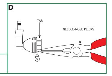
**5:** The accessory shade must fit snugly onto the slotted shade holder. If adjustment is necessary, carefully bend the slotted shade holder tabs slightly in or out with needle-nose pliers.
