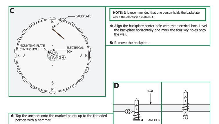
**7:** Screw in the threaded portion of the anchors with a Phillips screwdriver.
