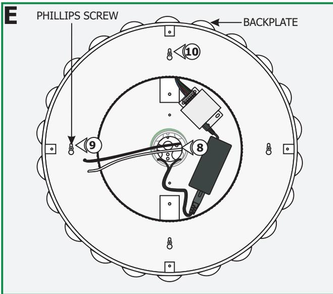
**8:** Feed the power wires coming from the electrical box through the backplate center hole.
