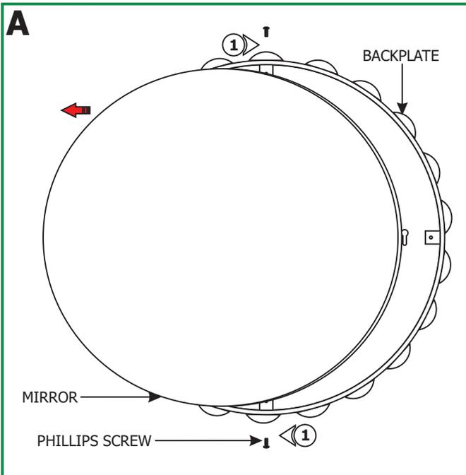
**1:** Remove the two Phillips screws from the sides of the backplate.
