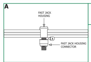
1: Place the Fast Jack housing onto the Monorail and use fingers to tighten the Fast Jack housing connector to the Fast Jack housing. Make sure that the Fast Jack housing connector is not cross threaded.
