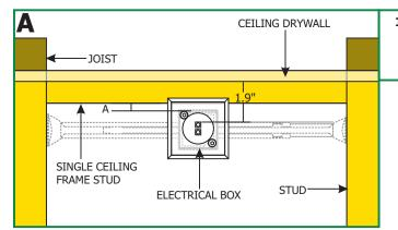
1: For Single Ceiling Frame Stud, use the Monorail 2" standoff to mount the Feed-End Power Canopy closest to the ceiling. Refer to the chart below to determine the 2" electrical box distance from the ceiling frame stud.
