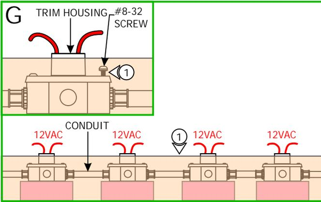
1: Align and secure the each trim housing to the octagon electrical box holes with the two #8-32 screws (not provided).
