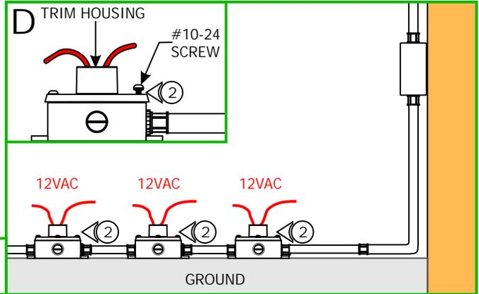
2: Align and secure each trim housing to the electrical box holes with the four #10-24 water sealant screws provided.
