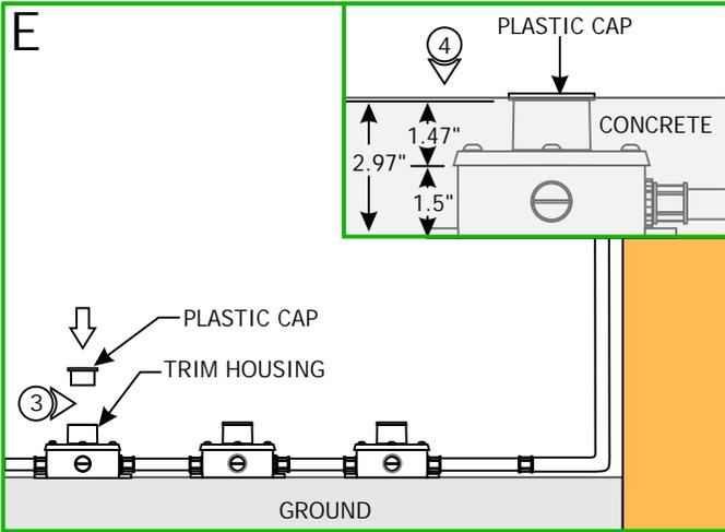
3: Insert the provided plastic caps to all trim housings to prevent particles and concrete debris from entering inside the box.
