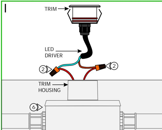
**NOTE:** For outdoor installation, use water proof outdoor wire nuts for power connection.
