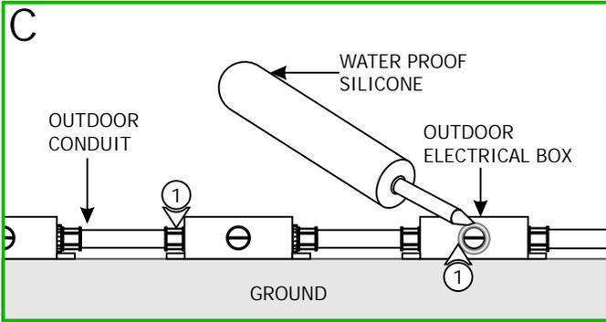
1: Caulk all areas of the outdoor electrical boxes and the conduit connectors with a water proof silicone to prevent water entering in the electrical boxes.
