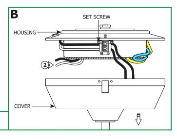
**2:** Unhook the transformer cover from the set screw and remove it from the transformer housing.
