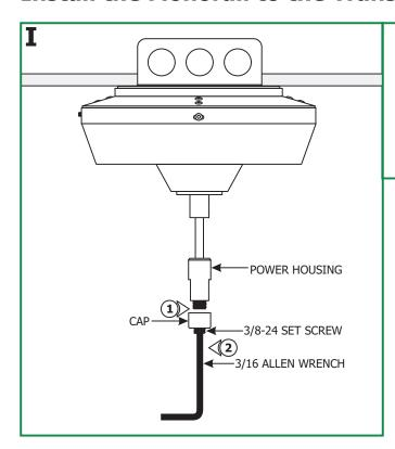
**NOTE:** The proper size standoffs should be installed to support the Monorail while connecting Monorail to the surface mount transformer (refer to the instruction provided with the standoffs).
