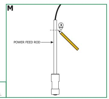
**3:** From the end of the power feed rod mark the rod to the amount that needs to be shorten. For example to resize 24" standoff to 17", mark 7" from the end of the power feed rod.
