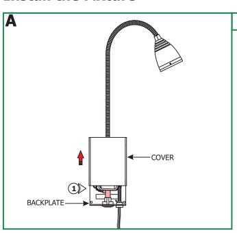
2: Hold the backplate against the surface where the fixture is going to be mounted. Level the backplate vertically and mark
