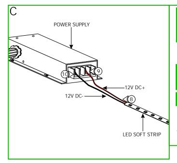
NOTE: In order to use small gauge wires from the power supply to the Soft Strip, it is recommended to install the power supply as near as possible to the LED fixture. See "Low Voltage Wire Size Chart" on page below.
