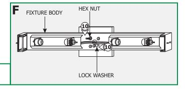
**10:** Secure the fixture body to the crossbar assembly by tightening the hex nuts and lock washers.
