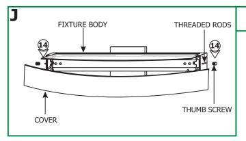
**14:** Replace the cover and tighten the two thumb screws to the threaded rods to secure the cover in place.
