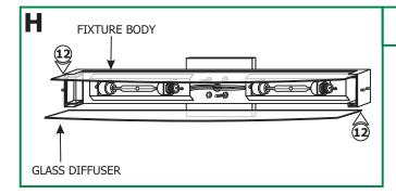
**12:** Insert the glass diffusers between the fixture body and inner bracket.
