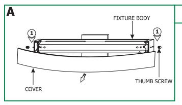
**1:** Remove the two thumb screws on the sides of the fixture body to detach the cover.
