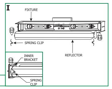
**13:** Align and insert the reflector ends into the inner bracket and secure it in place by replacing the spring clips.
