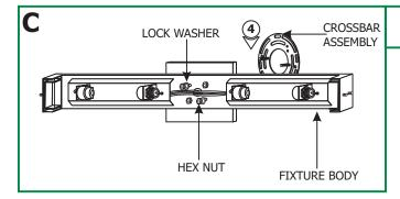
**4:** Loosen and remove the two hex nuts and lock washers from the center of fixture body to remove the crossbar assembly.
