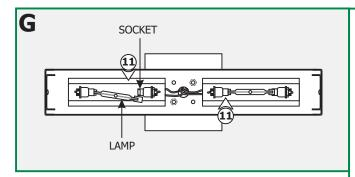
**<u>CAUTION</u>**: To reduce risk of a burn or electrical shock during lamping, disconnect the power to the fixture.
