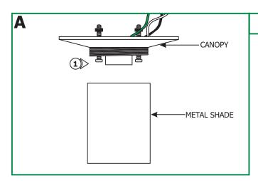
1: Loosen and remove the metal shade from the canopy.
