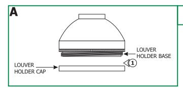
**1:** Unscrew and remove the louver holder cap from the louver holder base.
