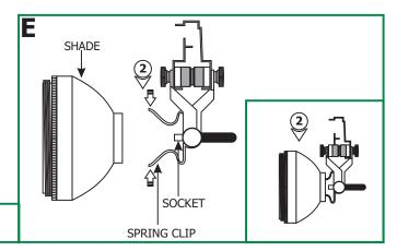
**2:** Squeeze the spring clip ends while inserting it into the shade.
