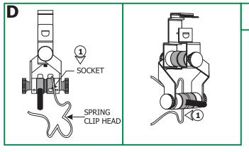
**1:** Push the spring clip completely onto the center of the socket groove until it snaps into place.
