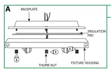
**1:** Remove the three thumb nuts from the threaded studs and detach the backplate from the fixture housing.
