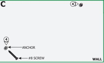
**4:** Tighten (not completely) the #8 screws into the anchors leaving the head unscrewed for 1/8".
