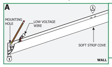
**NOTE:** Prior to Soft Strip Cove installation the low voltage wires should be present. Refer to the instructions provided with the power supply to install the low voltage wires before proceeding with the steps below.
