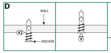
**NOTE:** Omit the steps 9 and 10 if installing to a wood surface.
