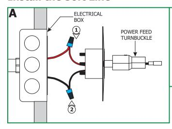
**NOTE:** The low voltage wires should be present in the electrical box. Refer to the instructions provided with the power supply to install the low voltage wires before proceeding with the steps below.
