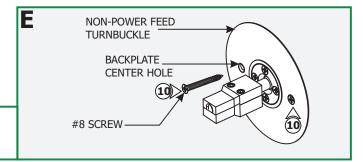
**10:** Push the non-power feed turnbuckle into the 1.8" cutout hole. Align the holes with the turnbuckles and secure it in place with the two #8 screws.
