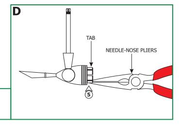
**5:** The accessory shade must fit snugly onto the slotted shade holder. If adjustment is necessary, carefully bend the slotted shade holder tabs slightly in or out with needle-nose pliers.
