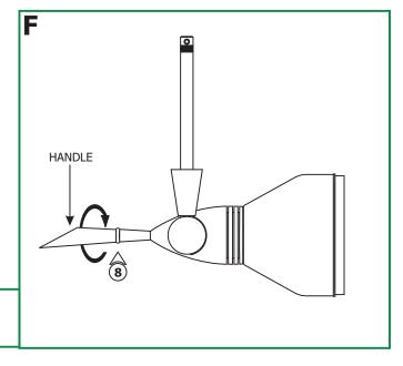
**8: OPTIONAL:** To position the handle in a different angle turn the plastic portion of the handle clockwise until desired position is achieved.
